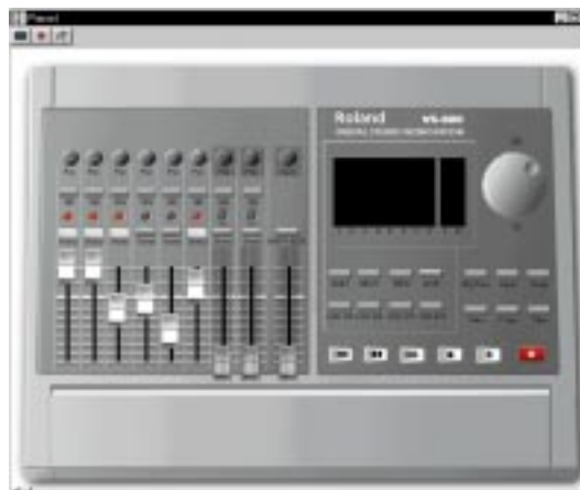
Fig 1 Cakewalk's StudioWare provides on-screen panels for synths and digital audio workstations like the Roland VS-880
